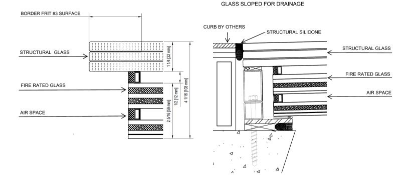
60 1/4" Max O.D. GLASS FRAME / STRUCTURAL GLASS 57 1/8" 2 HR. FIRE RATED GLASS
